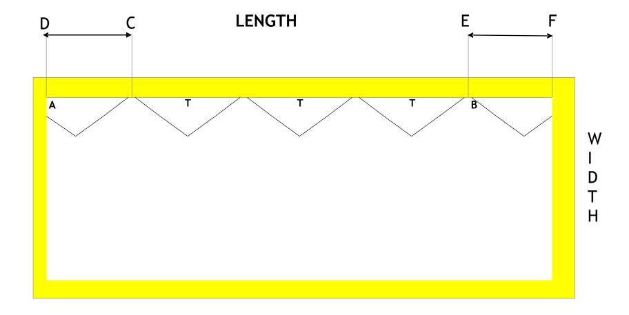
Cutting Triangle A Measure the dimension CD and cut the triangle to size along DE
